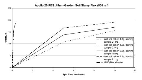
**Note:** Apollo 20 PP .45 $\mu$ m is a hydrophobic membrane and will normally require a minimum 2000 rcf to overcome the breakthrough pressure and develop a reasonable flow for most aqueous samples. (spun 5 minutes @ 2000rcf with MilliQ Biocel water = ~ 18 mL of filtrate) Reasonable flows can be achieved using lower rcf if the membrane is pre-wet with an organic solvent such as isopropyl alcohol.
